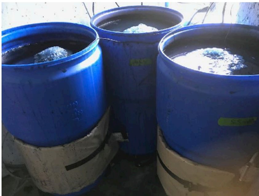
Three 14 gallon drum for indigo vats. Two of the vats are wrapped in a bucket heater band
